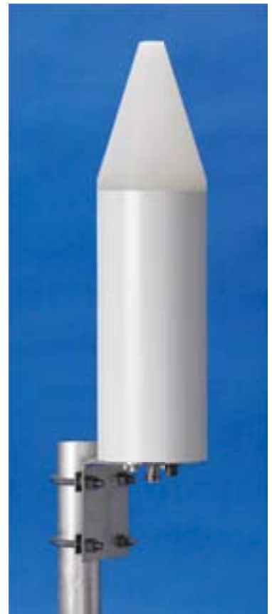
CPO235-4.5-R/QHO230-R combination antenna, with single RF connector and DC control connector. The antenna has an internal PIN diode RF switch.
