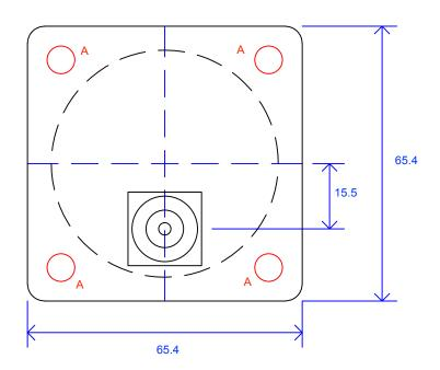
4 holes, A, 6.6 through equispaced on 69.9 PCD.
