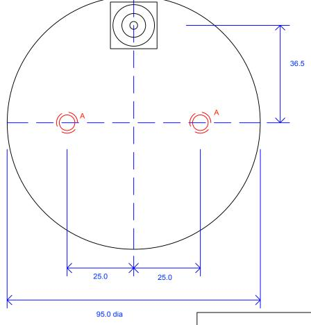
2 holes, A, with 5/16 - 18 X 1D blind helicoil insert.
